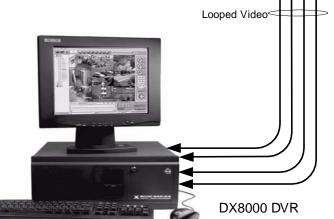
Coaxitron® Controlled PTZs can be controlled by a matrix bay and the DVR when the coax cable is looped from one device to another. In this example, the video is being looped from the matrix bay but it could also be looped from the DX8000 and then into the matrix bay.
