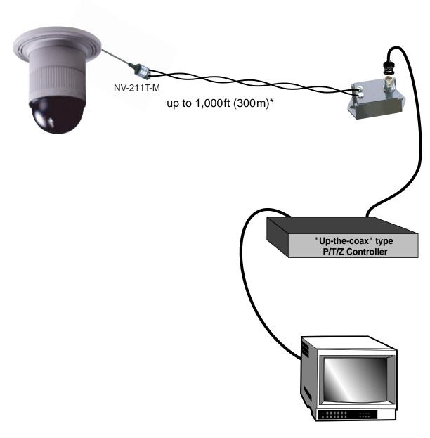
\* For digital recording applications it is recommended that Passive to Passive transmission distances be limited to no more than 750 ft. For distances greater than 750 ft please use an NVT Active Receiver product.
